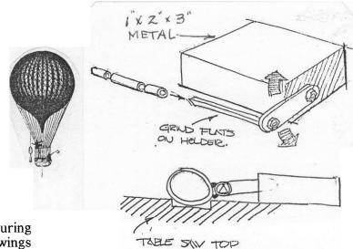
The above fixture was used by Will Fetherolf of Boise, Id. to align and hold the hinge bushings on the tail feathers while welding. The work was held in place on the top of his table saw.
